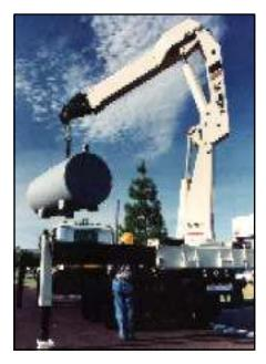
**Note:** Weights of all accessories attached to the boom or loadline of the crane must be deducted from the effective lifting capacity. Additional accessories not listed may be available. Not all accessories are available for all crane series, and some accessories cannot be used in combination with other accessories. Consult your dealer or the factory for accessory capabilities, availability and pricing.
